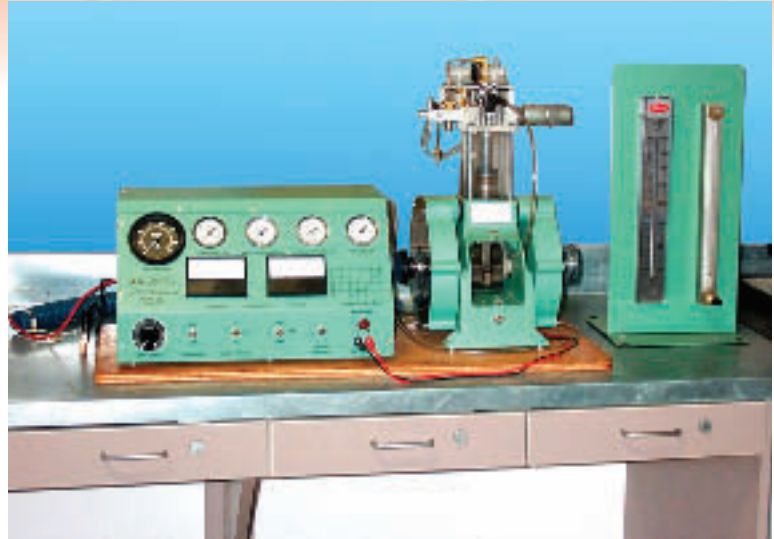
MEG150: Oil-less 4 cycle engine operates with any alternative fuel.
